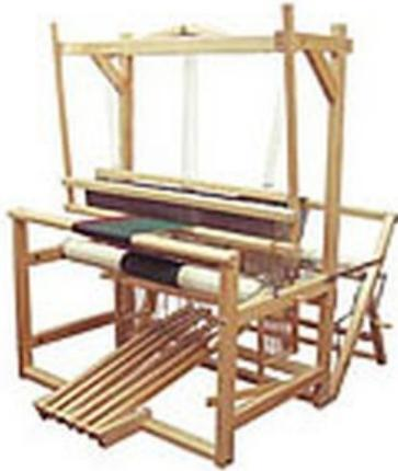
Comes complete with flying shuttle beater with a 12 dents per inch reed. The loom has many extras:
